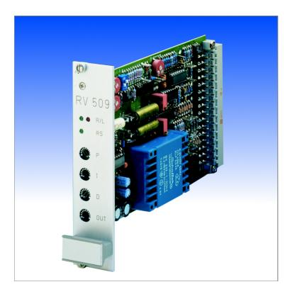
As a complement to our range of sensors and measurement amplifiers, we have engineered and built the RV 509 PID controller, used in constructing closed-loop control circuits.
