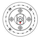
The **Cantilever sensor roll** with integrated force measurement can be installed just like an unilateral installed standard web guide roll without major mechanical modifications.
