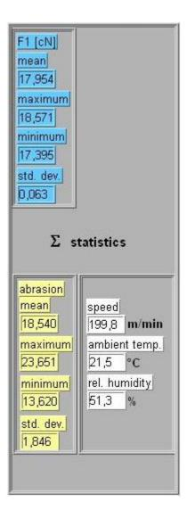
Once a measurement has run to completion the data captured for tensile forces  $F_1$  and abrasion will be evaluated statistically:
